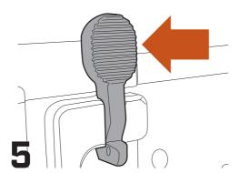
Once the loaded magazine is inserted, depress the bolt release on the left side of the receiver. The firing action is reactivated.
